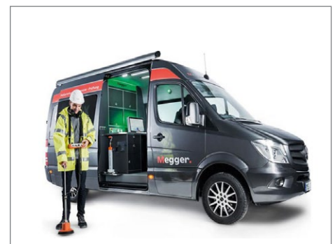
Figure 15: An example of a modern, customisable specification, cable fault location test van.
