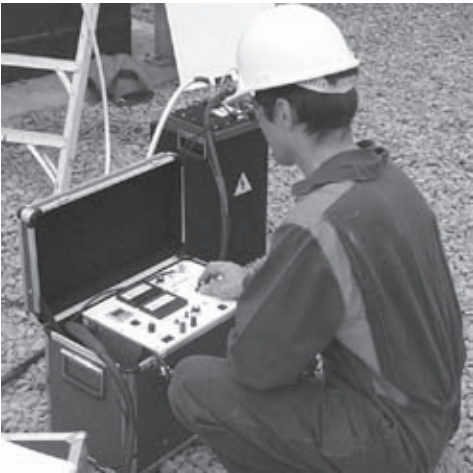
VLF Testing of an MV XLPE Cable Prior to Commissioning.
